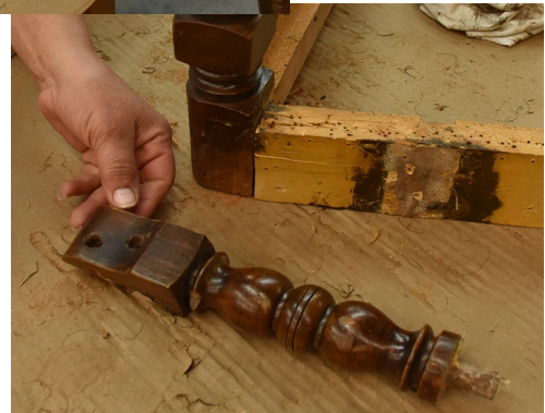
(3) Because of the many tack holes, a new frame piece will be added for support, the chipped spindle will be repaired before reassembly.
