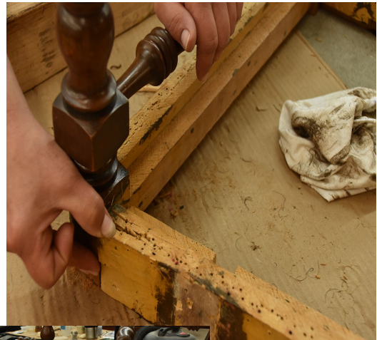
(3) Because of the many tack holes, a new frame piece will be added for support, the chipped spindle will be repaired before reassembly.
