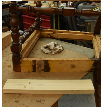
(3) Because of the many tack holes, a new frame piece will be added for support, the chipped spindle will be repaired before reassembly.
