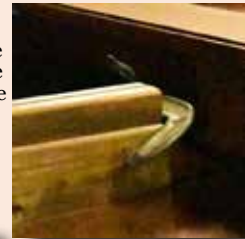
Below, the partitions are supported by one leg which provides the spacing needed for the structure to fit over the existing workspace dividers on the bench. Right, the structure is clamped onto the molding for stability.
