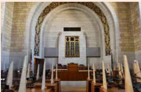
The Norris Legislative Chamber with the finished plywood and Plexiglas divider in place, above. Right, the dividers were designed by OCC staff to rest on the Senator’s desks without damaging the original walnut and leather surfaces.
