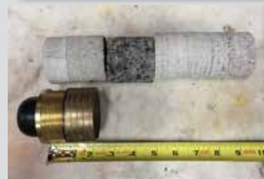
Core layers above from left to right, Napoleon Gray marble finish floor, setting bed, dark cinder fill for original conduit placement above five inches of concrete structural floor.
