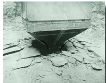
Recording the weight of the load at the point the sandstone failed provided information used by engineers to design proper footings and foundations for Goodhue's monumental Capitol.
