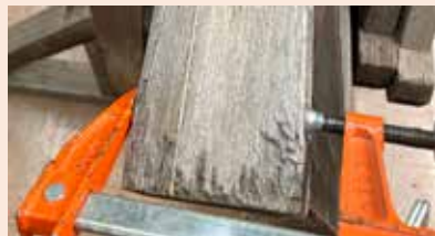
Left, the weathered barricades arrive in OCC Carpenter's Shop. The first step in the refurbishing process was to address cracks in the wood. Some cracks were stabilized with glue, above. Right, if the barricade was too weather damaged, deteriorated material was removed and replaced with new wood.
