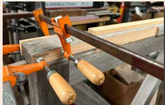
Left, the weathered barricades arrive in OCC Carpenter's Shop. The first step in the refurbishing process was to address cracks in the wood. Some cracks were stabilized with glue, above. Right, if the barricade was too weather damaged, deteriorated material was removed and replaced with new wood.
