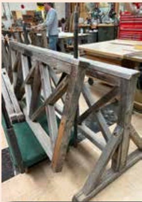
Left, the weathered barricades arrive in OCC Carpenter's Shop. The first step in the refurbishing process was to address cracks in the wood. Some cracks were stabilized with glue, above. Right, if the barricade was too weather damaged, deteriorated material was removed and replaced with new wood.
